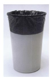
WB22 is a static dissipative, high impact, non-black wastepaper basket. This high-density polyethylene container does not contain carbon, dyes, or additives making it ideal for all applications demanding cleanliness. The trash barrel will not tribogenerate and will dissipate static electricity. The container measures  $10^8$  -  $10^{12}$  ohms for surface resistance.
